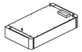
Beneath the BMS, you can stack 2-8 4.8kWh battery modules for a total capacity range of 9.6kWh to 38.4kWh. These battery modules are made from lithium iron phosphate (LiFePO4 or LFP), which is one of the safest lithium battery types.
